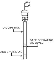
Figure 14. Engine Oil Dipstick
